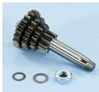
202.1417 Vespa 50/125 ET3 Z=10-14-17-20 Primary ratio-Primario
