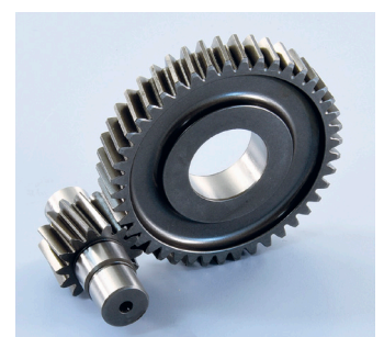
202.1414 Piaggio Liberty/Vespa 50 4T iGET Z=14/43 Secondary ratio-Secondario
