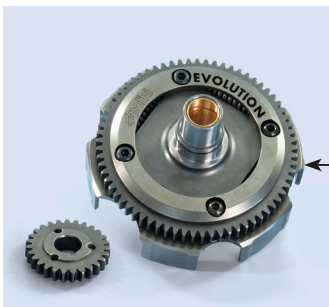
202.1221 Vespa 50 Z=24/72 Primary ratio-Primario
