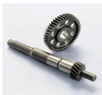
202.1412 Vespa 125 Primavera 4T Z=17/45 Primary ratio-Primario
