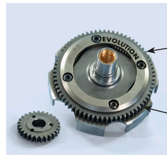
202.1222 Vespa 125 ET3 Z=27/69 Primary ratio-Primario
