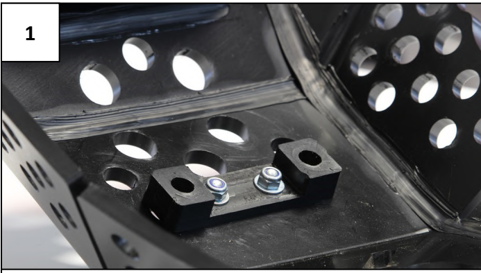
1 15mm plastic block + 2 Tfhc 6x20mm + 2 M6 Washers + 2 Em6f
