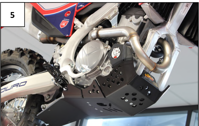
5 Fix the front with the 2 screws
